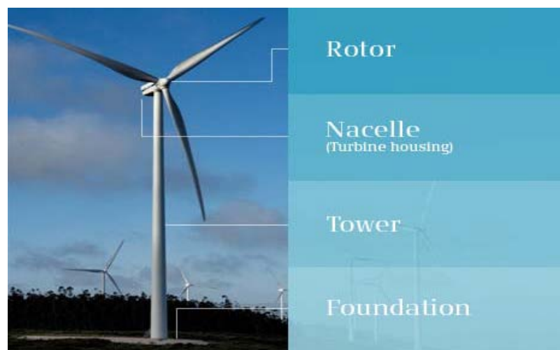
Figure 6: Anatomy of a Wind Turbine Generator
