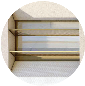
Aluminium sunshade screen detail (double screen)
