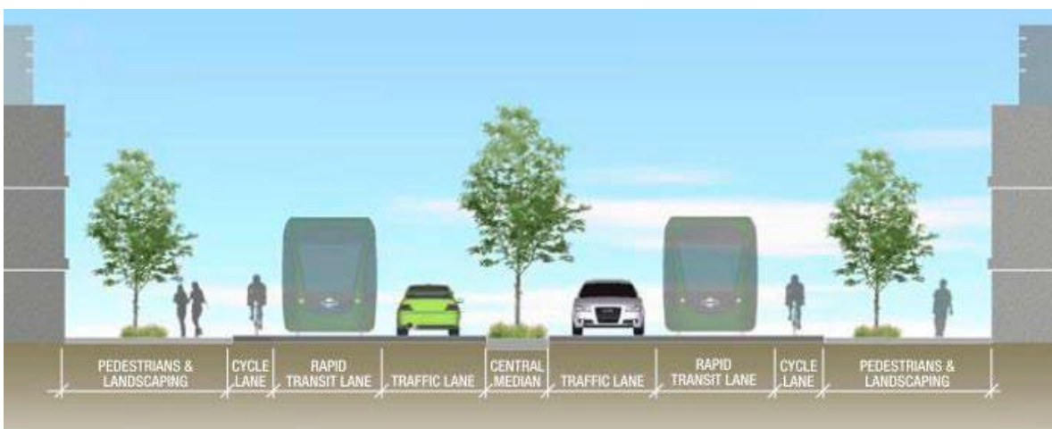
Figure 4-3 Indicative Cross Section - Public Transport Boulevard
