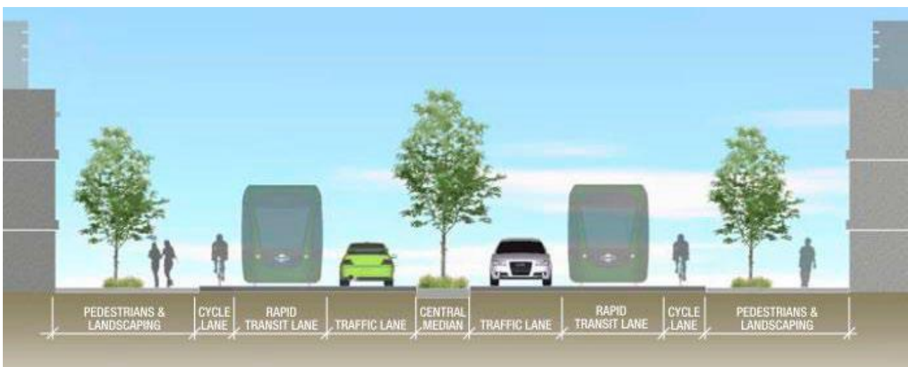
Figure 4-3 Indicative Cross Section - Public Transport Boulevard
