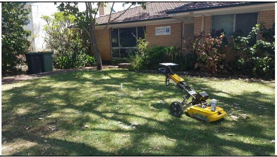
Photo 4. Locating of underground services by Ground Penetrating Radar (GPR)
