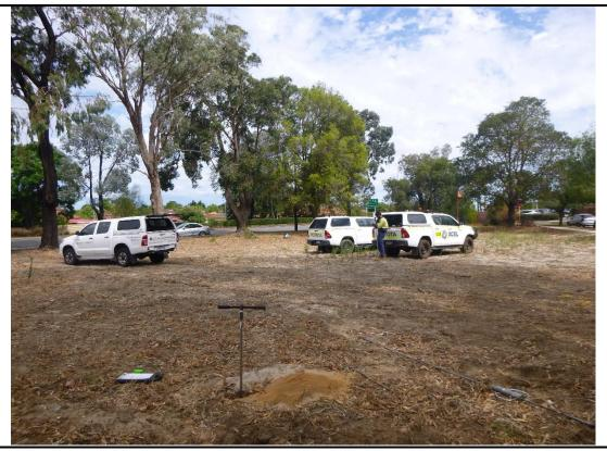
Photo 5. Test Location 02 (TH2), Sub-surface probing by using a hand auger
