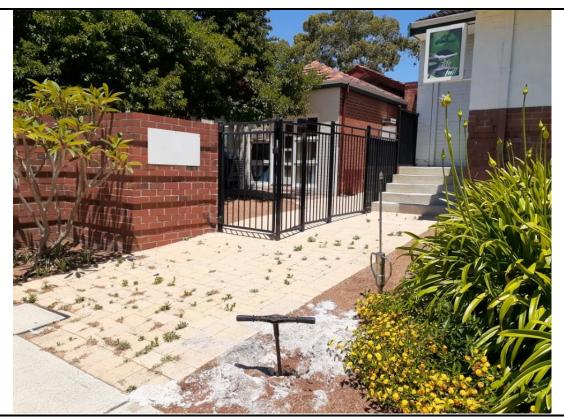
Photo 7. Test Location 03 (TH3), Sub-surface probing by using a hand auger and PSP testing
