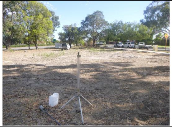
Photo 10. Soil permeability testing with a Guelph Permeameter (FPT1)
