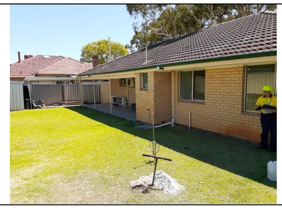
Photo 5. Test Location 02 (TH2), Sub-surface probing by using a hand auger and PSP testing
