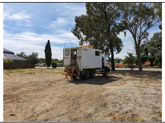
Photo 12. Testing Cone Penetration Test at Test Location, CPT2
