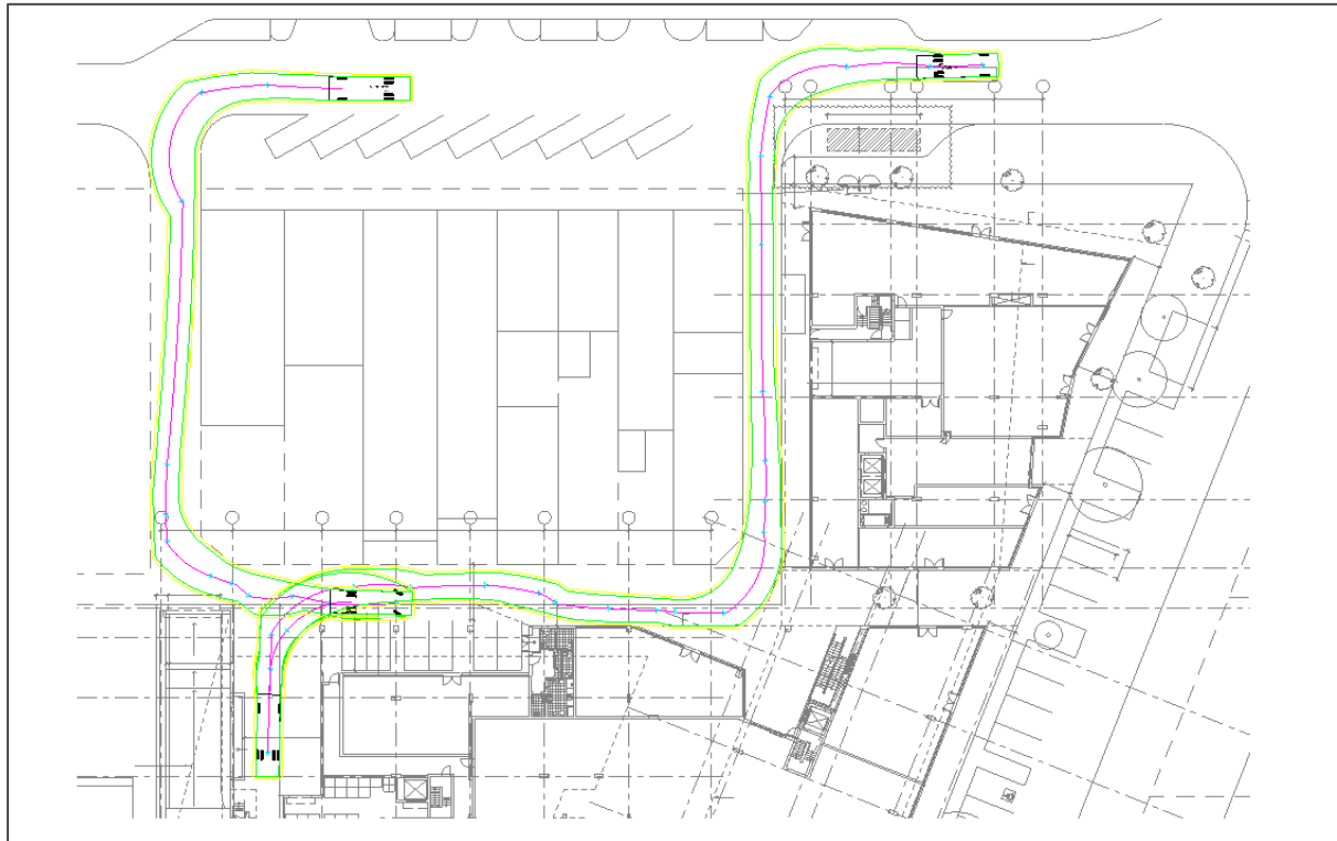
Diagram 2: Medium Ridged Vehicle (MRV) Waste Collection Swept Path
